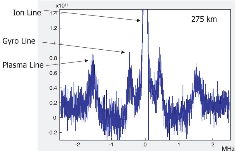
Fig. 1: Full incoherent scatter spectral measurements showing the ion line, gyro, and plasma line. Adapted from Aponte et al. [2007] but based on the measurements of Bhatt et al. [2006].
