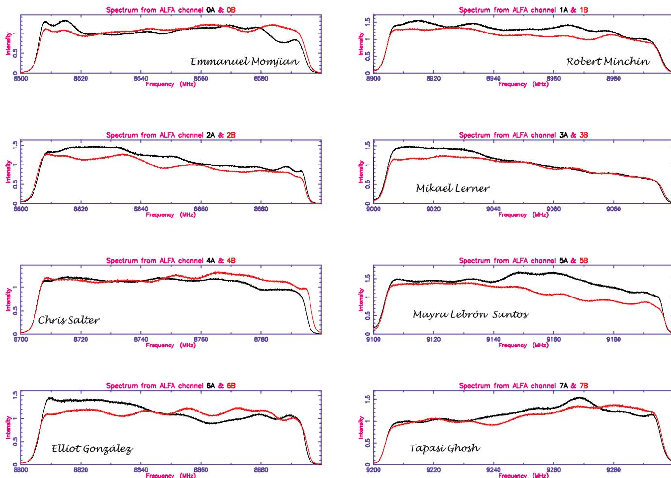
Fig. 22: First scientific light for the WAPP dual board capability. The diagram shows bandpass curves (two polarizations) for the eight 100-MHz bands covering 8500-9300 MHz observed with the X-band receiver during the first night of dual-board observing. The labels incorrectly say “ALFA beams”, since the ALFA quick-look display was used to create this figure. The diagram also bears the names of the staff members participating in the observation. [Courtesy: M. Lerner]
