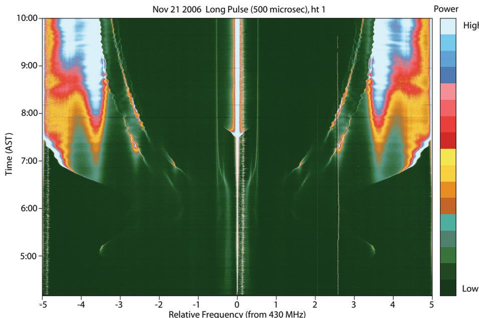
Fig. 6: Dawn time spectra obtained for an altitude of 140 km on Nov 21, 2006. The appearance of the plasma line at  $\sim$  1 MHz is due to the sunrise at this altitude at 05:47 AST. (Courtesy: M. Sulzer)
