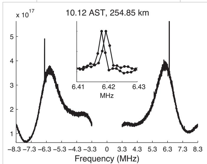
Fig. 2: Example of full plasma line spectrum measured on April 1, 2006. The y axis corresponds to un-normalized power. The inset is a zoomed-in plot of the normalized peak with the down-shifted line folded over to positive frequencies. From Nicolls *et al.* [2006]
