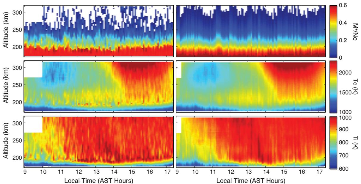
Fig. 4: Results from height-by-height fits (left) and fits with hyperbolic tangent model (right). For each side, the top panel is molecular ion fraction, the middle panel is the electron temperature, and the bottom panel is the ion temperature. From *Aponte et al.* [2007].
