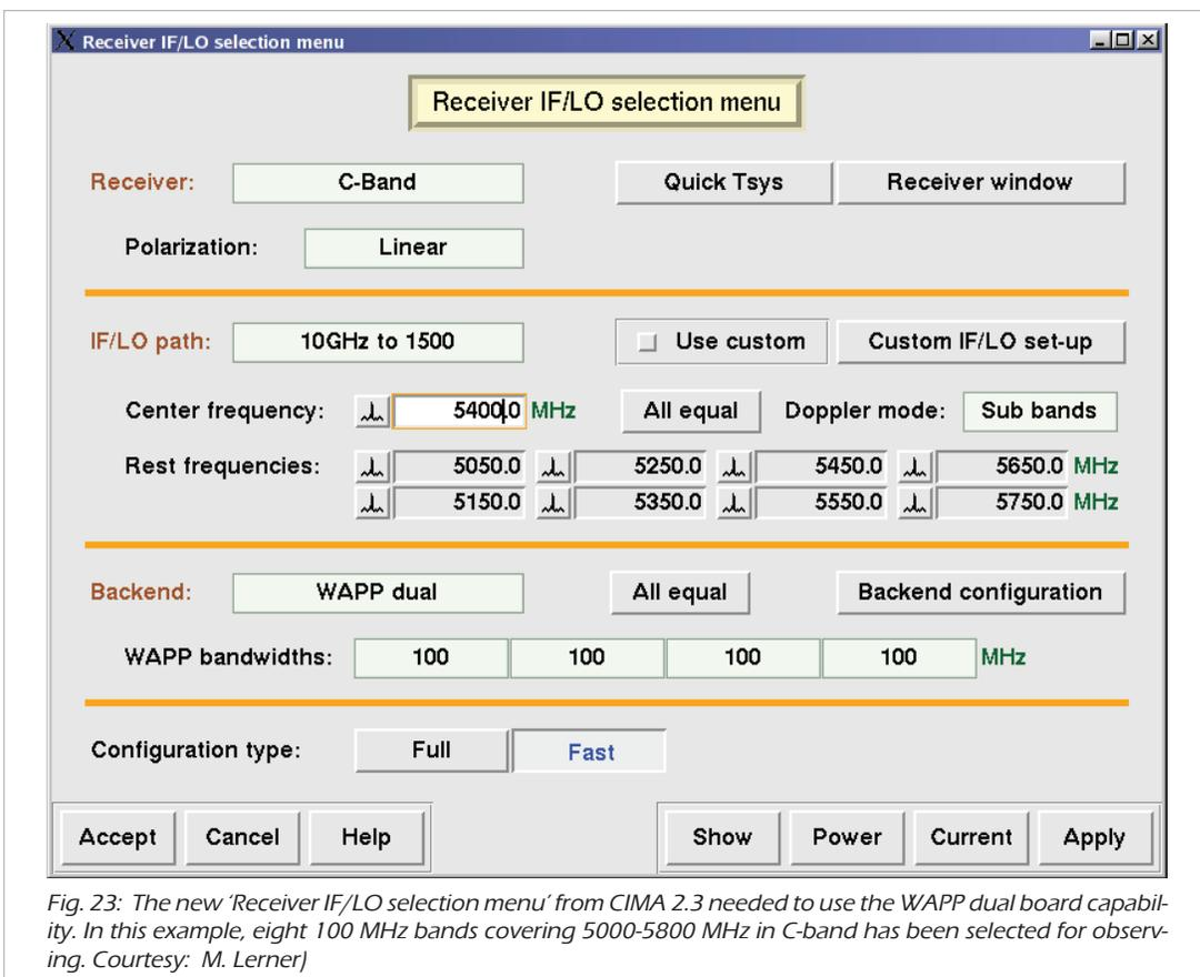
Fig. 23: The new 'Receiver IF/LO selection menu' from CIMA 2.3 needed to use the WAPP dual board capability. In this example, eight 100 MHz bands covering 5000-5800 MHz in C-band has been selected for observing. Courtesy: M. Lerner)
