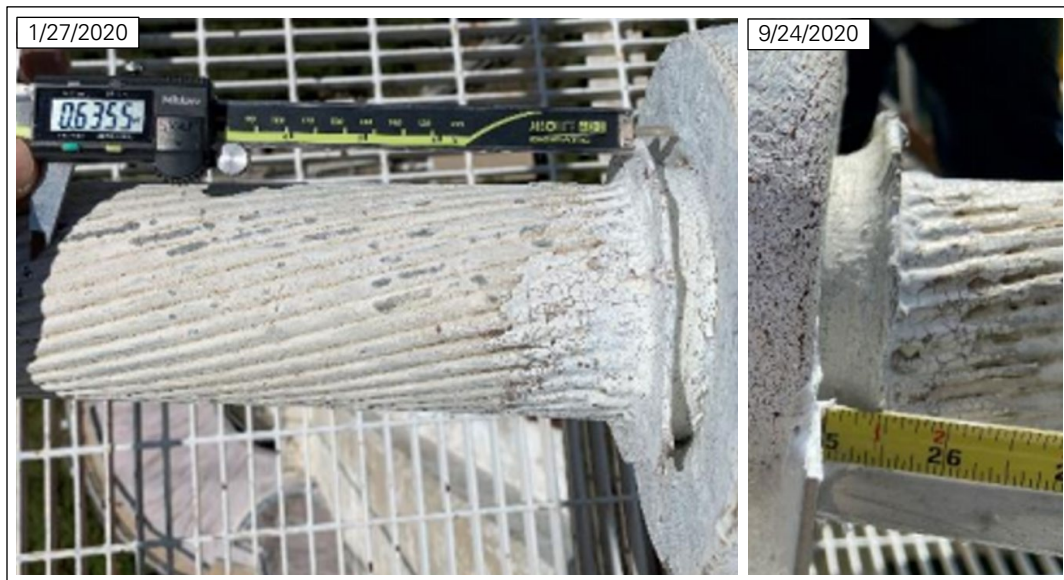
Figure 25: Cable slip at socket M12W_T (left photo: NAIC Arecibo Observatory, a facility of the NSF; right photo: WJE 12 ).
