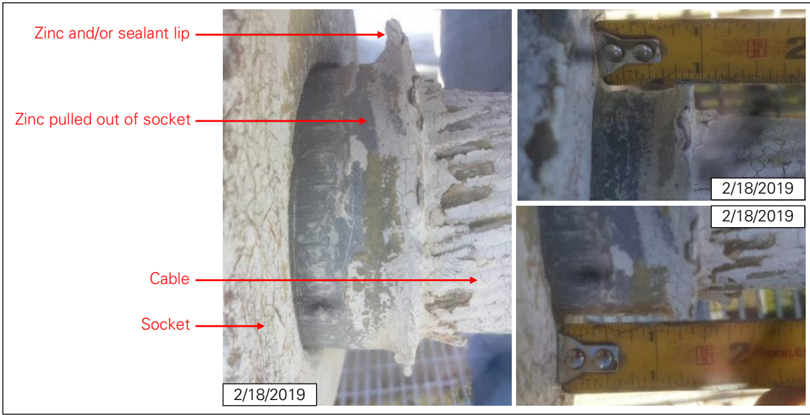
Figure 18: Cable slip at socket M4N_T. As seen from the north side (left) and measured on north (top right) and south (bottom right) sides of socket (photos: NAIC Arecibo Observatory, a facility of the NSF).
