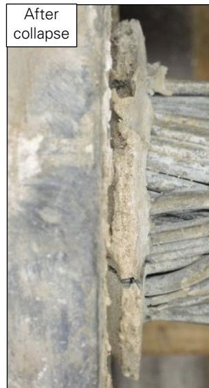
Figure 29: Cable slip at socket M8S_P.
