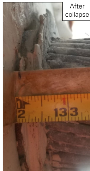
Figure 40: Cable slip at socket B8N_G.
