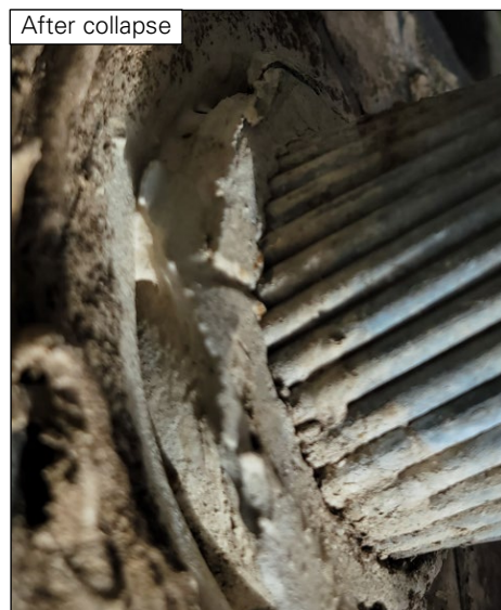
Figure 28: Cable slip at socket M8N_P.
