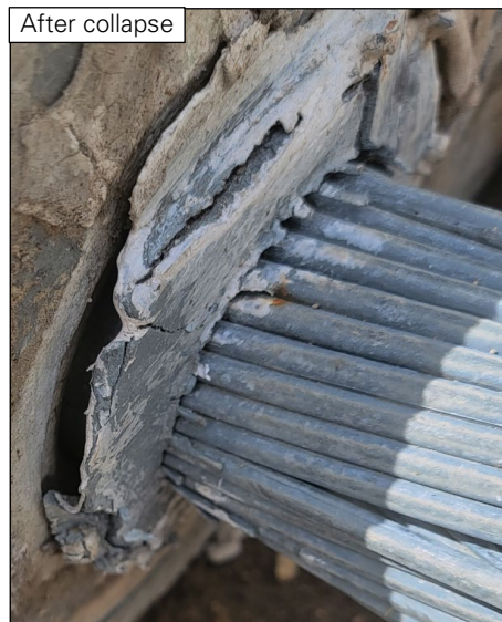
Figure 30: Cable slip at socket M12E_P.
