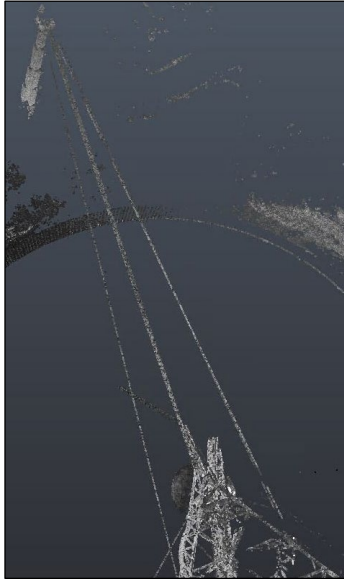
Figure 1: Tower 8 mains in August 2020 laser scan.
