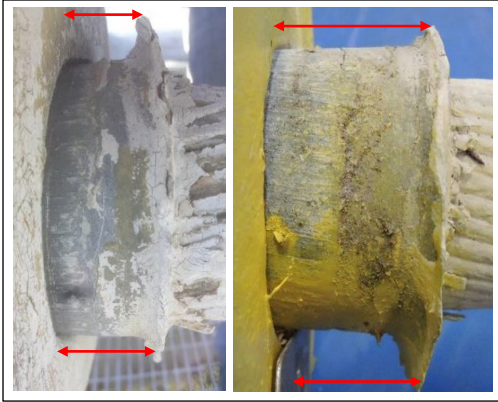
Figure 16: Cable slip at socket M4N_T (left) and B12W_G (right) (photos: NAIC Arecibo Observatory, a facility of the NSF).
