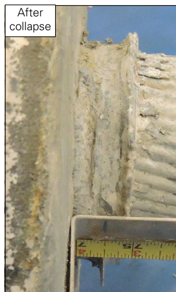
Figure 39: Cable slip at socket B4S_G.
