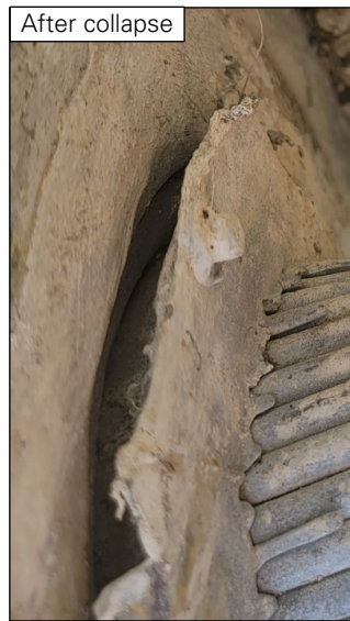
Figure 31: Cable slip at socket M12W_P.
