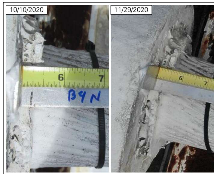
Figure 32: Cable slip at socket B4N_T (left photo: WJE 13 ; right photo: NAIC Arecibo Observatory, a facility of the NSF).
