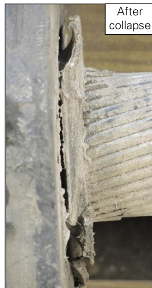
Figure 27: Cable slip at socket M4S_P.
