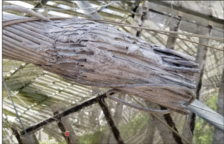
Figure 3: Cable end pulled out of socket M4N_T.
