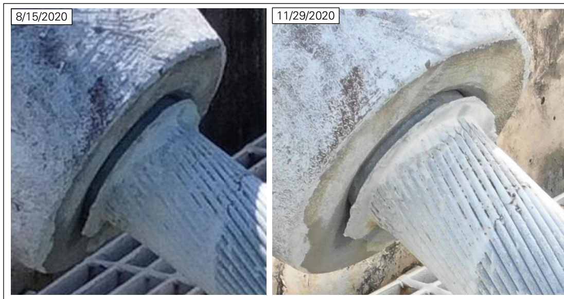
Figure 34: Cable slip at socket B8N_T (photos: NAIC Arecibo Observatory, a facility of the NSF).
