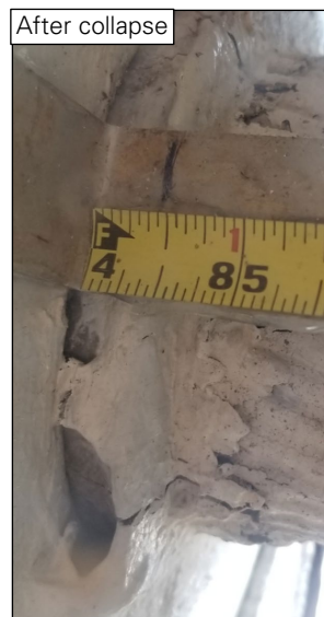
Figure 41: Cable slip at socket B8S_G.
