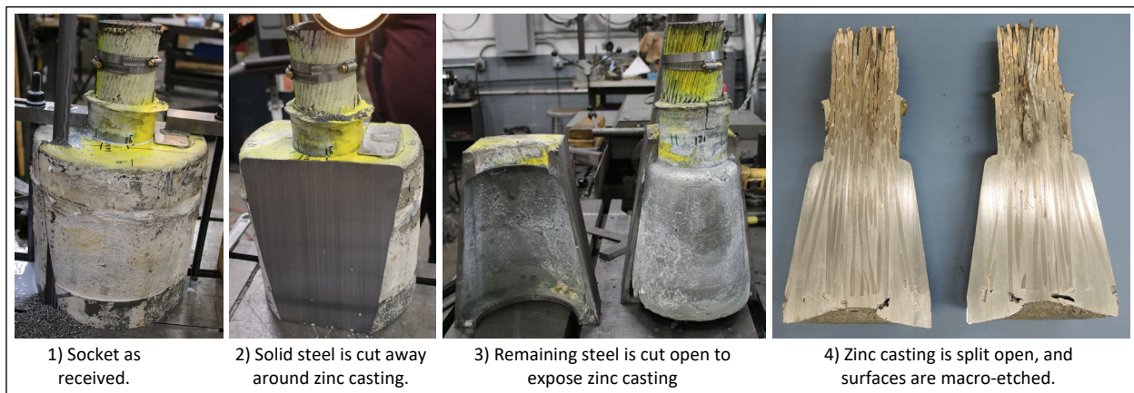
Figure 10: Initial processing of socket B12W_G (photos: Socotec).
