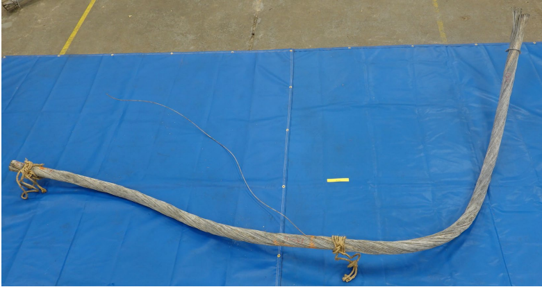
Figure 3: Intact segments of four M4 cables (photos: Socotec).
